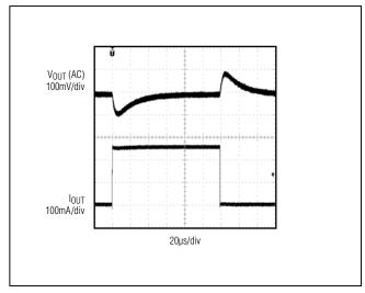
Figure 7. MAX17501F No Load to 250mA Load Transient
