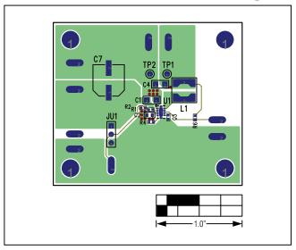
Figure 12. MAX17501B/MAX17501F EV Kits PCB Layout—Component Side
