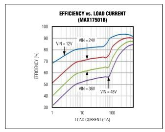
Figure 3. MAX17501B Efficiency
