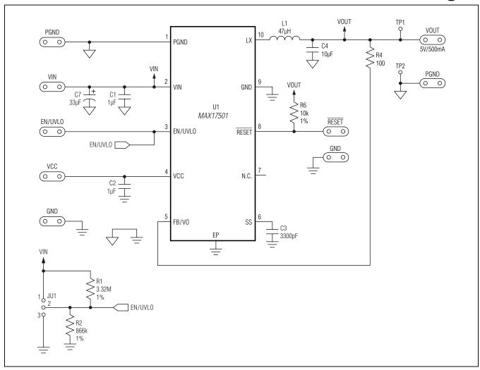
Figure 9. MAX17501B/MAX17501F EV Kits Schematic
