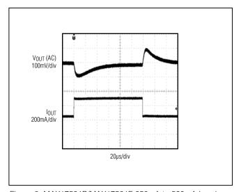
Figure 8. MAX17501B/MAX17501F 250mA to 500mA Load Transient
