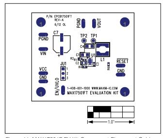
Figure 11. MAX17501F EV Kit Component Placement Guide—Component Side
