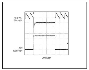
Figure 6. MAX17501B 5mA to 255mA Load Transient
