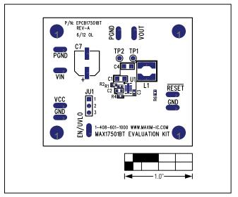
Figure 10. MAX17501B EV Kit Component Placement Guide—Component Side
