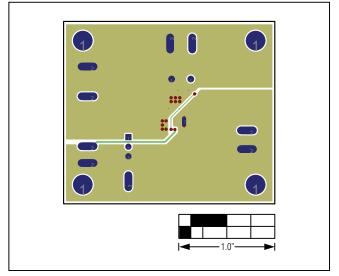
Figure 13. MAX17501B/MAX17501F EV Kits PCB Layout—Solder Side
