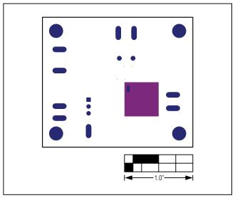
Figure 15. MAX17501B/MAX17501F EV Kits PCB Layout— Bottom Solder Mask
