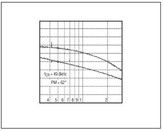
Figure 5. MAX17501B/MAX17501F Full-Load Bode Plot (VIN = 24V)
