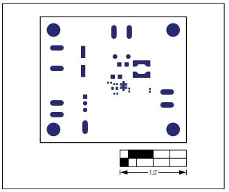
Figure 14. MAX17501B/MAX17501F EV Kits PCB Layout—Top Solder Mask
