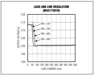
Figure 1. MAX17501B Load and Line Regulation
